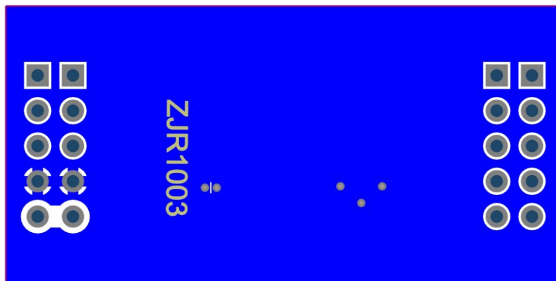
Figure 29. ZJR1003 Evaluation Board Layout (Bottom Layer)
