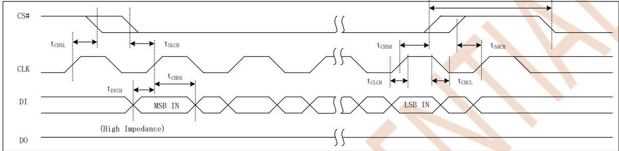
Figure 8.5 Input Timing
